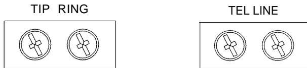
These inputs are balanced with no ground connection, since simple twisted-pair is the intended hook-up cable.
